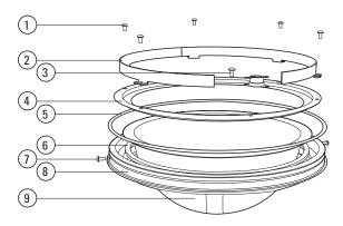
Figure 3. Exploded Assembly Diagram, Pendant Lower Dome
